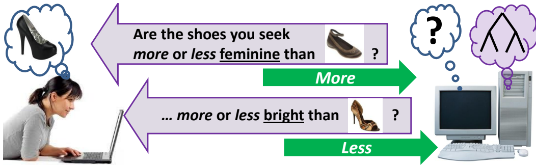
Figure 1.2: The active version of WhittleSearch requests feedback in the form of visual attribute comparisons between the user’s target and images selected by the system. To formulate the optimal question to ask next, it unifies an entropy reduction criterion with binary search trees in attribute space.
