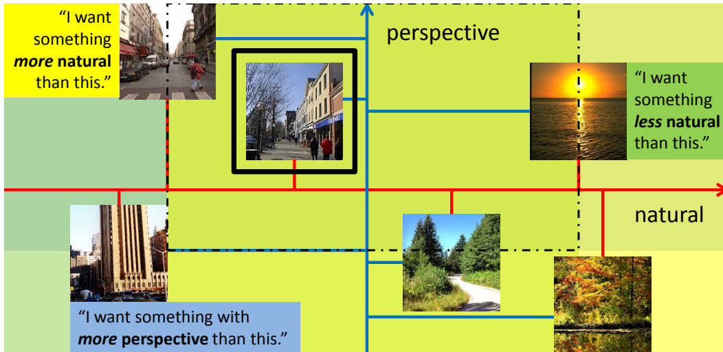
Figure 3.2: A toy example illustrating the intersection of relative constraints with M = 2 attributes. The images are plotted on the axes for both attributes. The space of images that satisfy each constraint are marked in a different color. The region satisfying all constraints is marked with a black dashed line. In this case, there is only one image in it (outlined in black). Best viewed in color.
